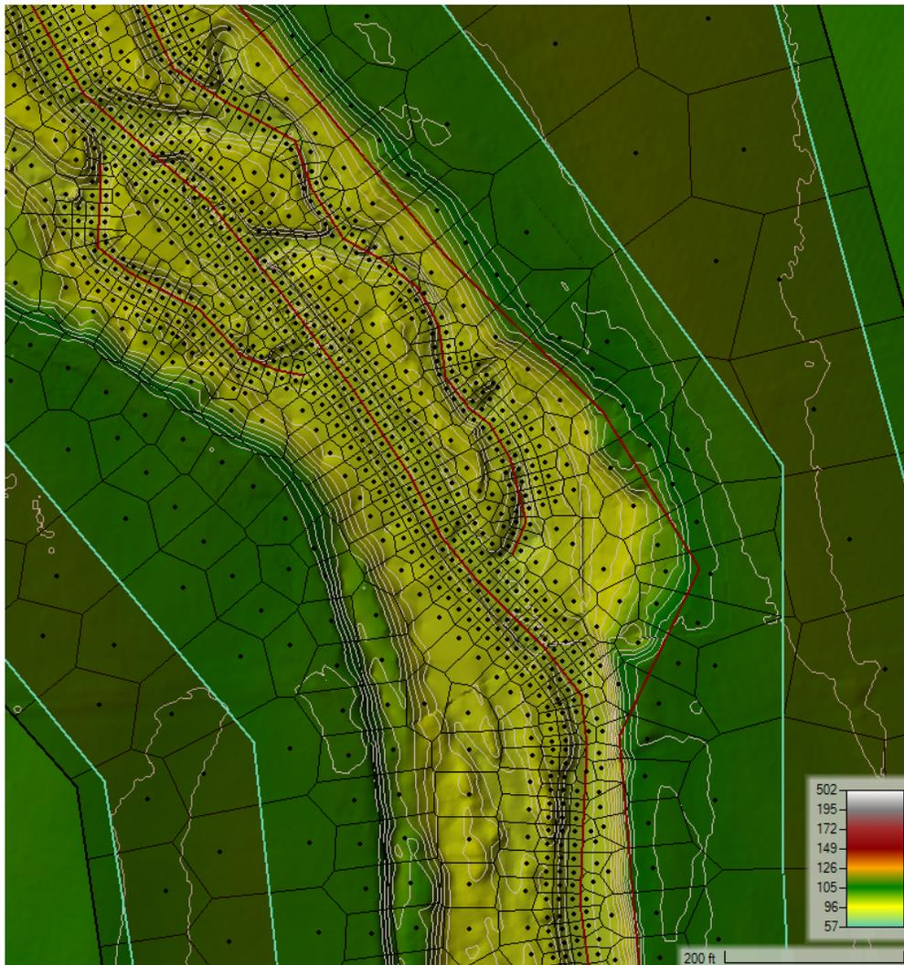
*Figure 9. Model mesh grid and computation points, shown on underlying terrain with 2 ft contours. Breaklines (maroon lines) used to align computation points with flow and refinement regions (shaded olive areas) used to reduce point density on infrequently inundated areas. Map units in ft from unit system used in HEC-RAS.*
