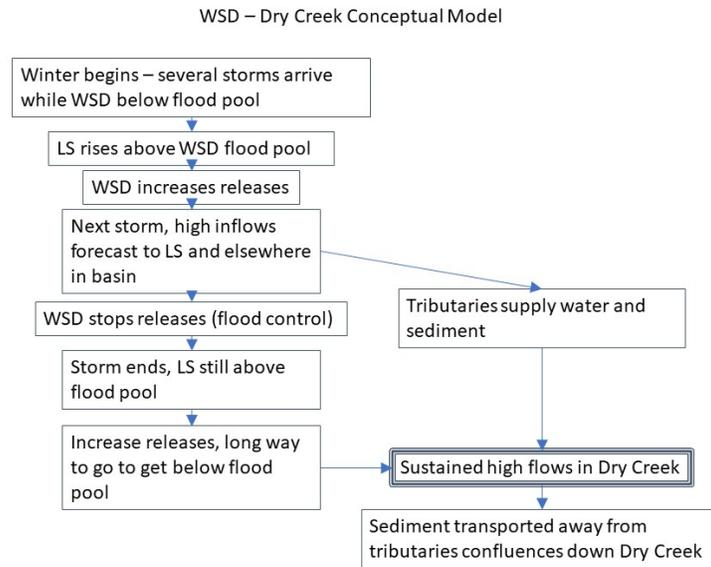
Figure 5. Conceptual model of how sustained high flows in Dry Creek lead to sediment transport away from tributary confluences and into restoration sites.
