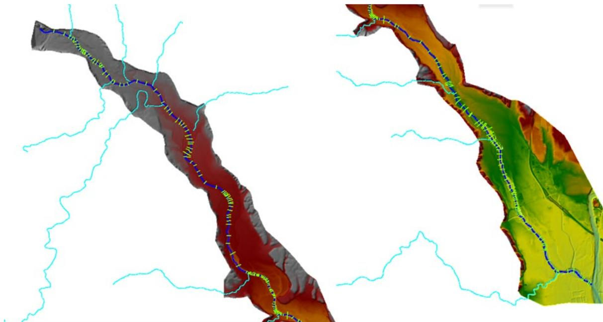
*Figure 7. Modeling domain with cross sections shown in green and tributaries shown in light blue. Left-hand side is the upstream portion of the model, and right-hand side is the downstream portion.*
