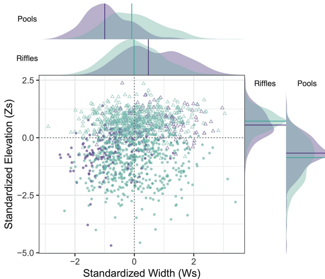
Figure 2. Distribution of field-identified pools (circles) and riffles (triangles) in terms of standardized width and elevation as well as velocity reversal (purple) and no velocity reversal (teal) locations. Purple and teal solid lines represent median standardized width and elevation for pools and riffles under velocity reversal and no velocity reversal conditions.
