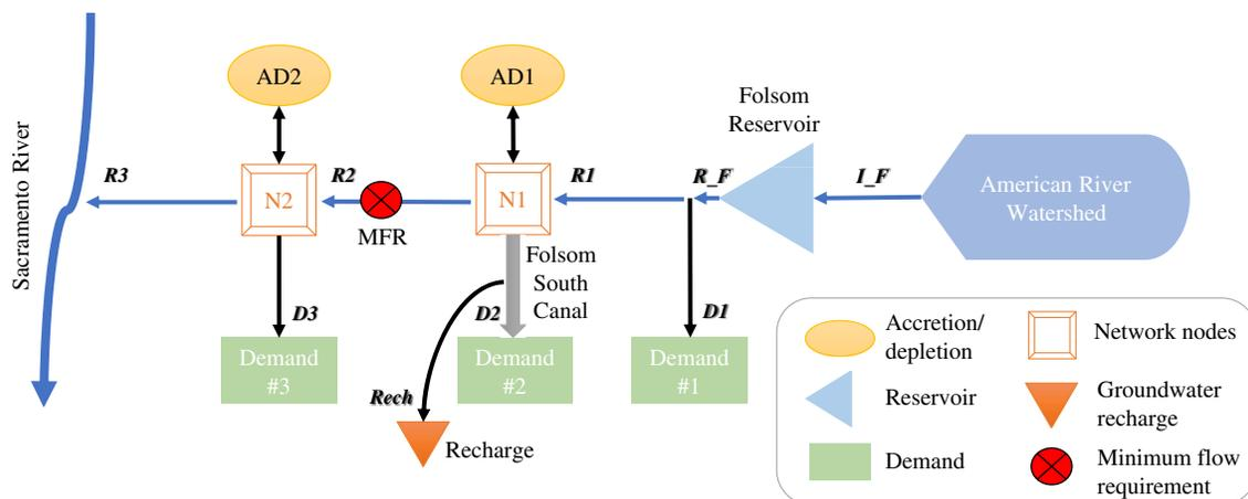
**Fig. 3.** American River water system schematic in FolSim.
