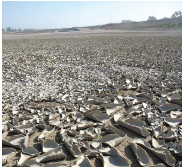
Figure 20 Accumulated clogging layer from a recharge basin operated by OCWD. from Figs. 5–12 O. C. W. District. Orange county water district groundwater management plan 2015 update, Tech. rep. June 2015. https://www.ocwd.com/what-we-do/groundwater-management/groundwater-management-plan/ .
