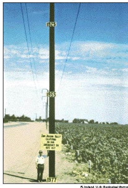
Figure 3. Historical land subsidence observed in the Central Valley near Mendota, California (USGS 2000).
