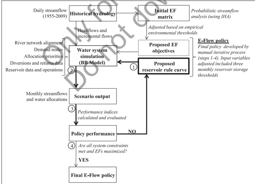
Figure 2. Study method framework, including key inputs and outputs of linked major components (boxed) and computations performed (indicated by italics)
