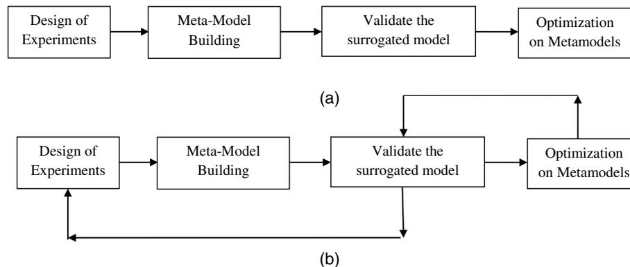
Fig. 2. Metamodel-based design optimization: (a) sequential structure; and (b) adaptive structure. (Adapted from Wang and Shan 2006.)
